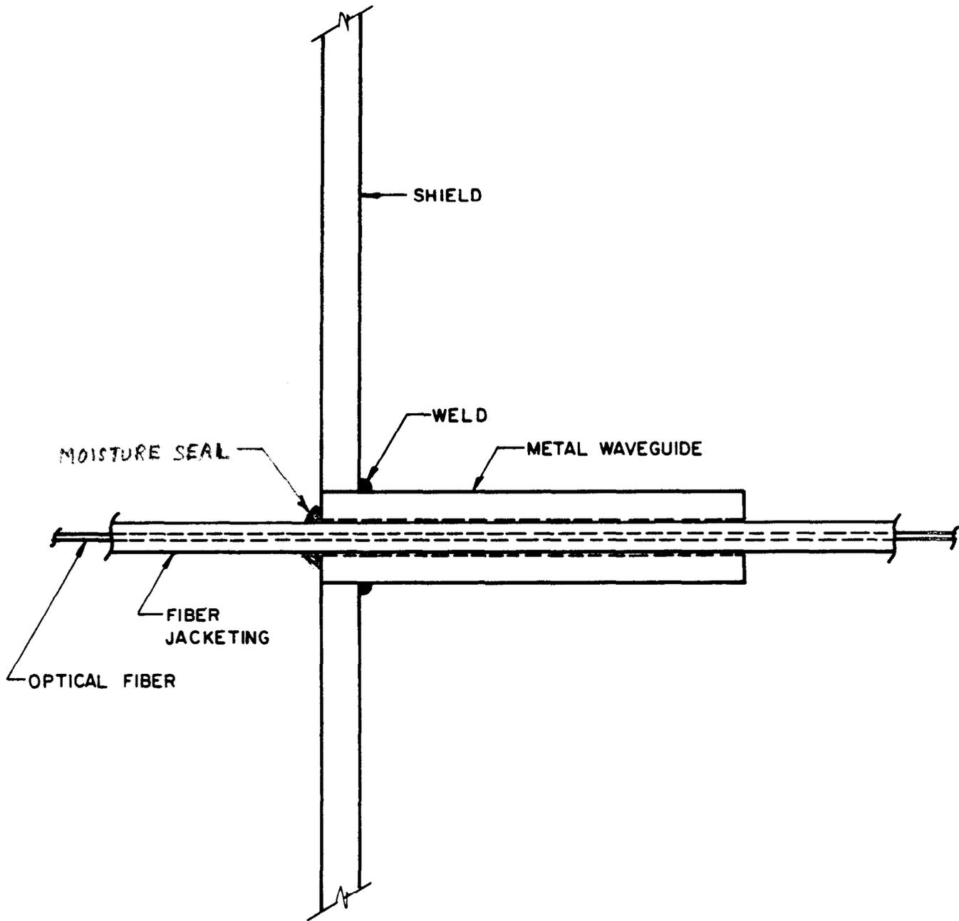
Figure 3-6. Optical fiber shield penetration.
