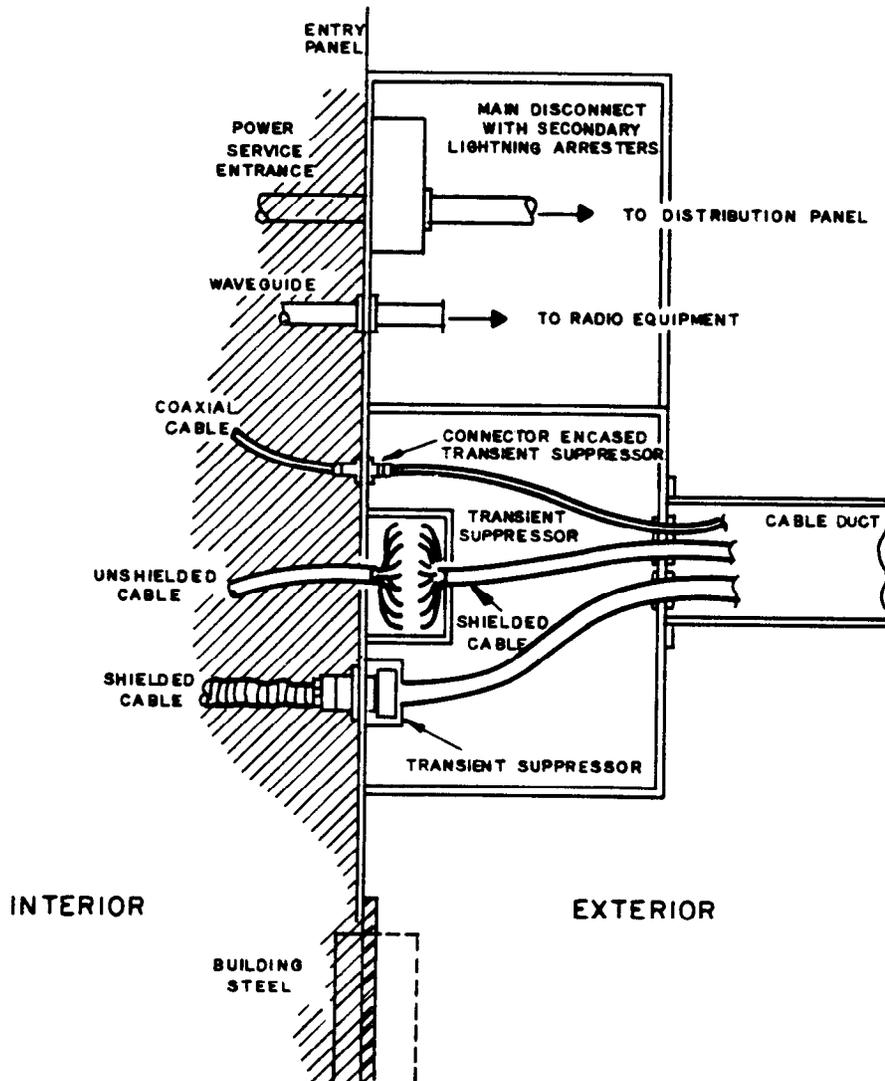
Figure 3-5. Shielded enclosure: cable entry vault.
