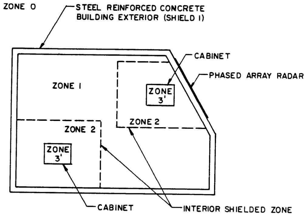
Figure 3-4. Zonal shielding concept with steel-reinforced concrete as shield 1.
