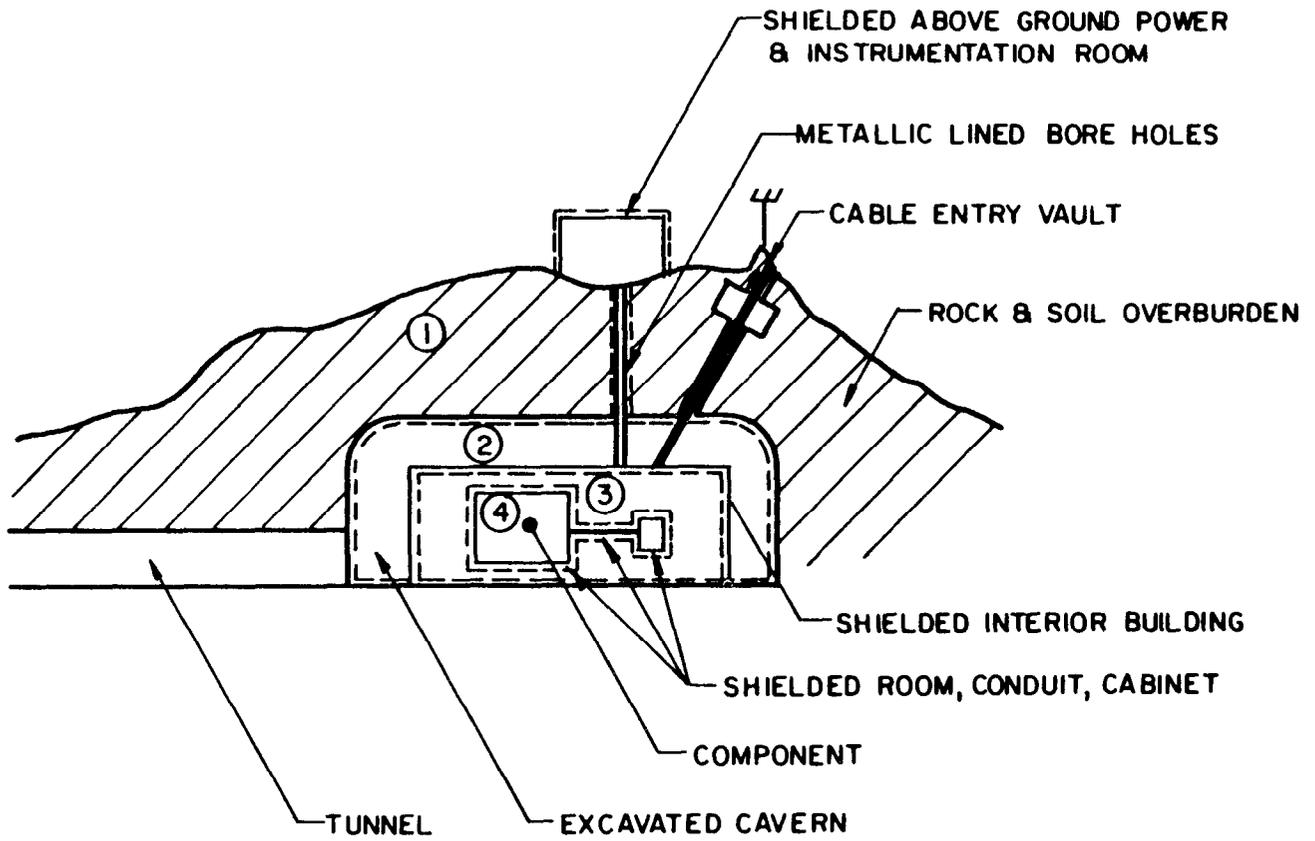
Figure 3-3. Underground facility with four zones.
