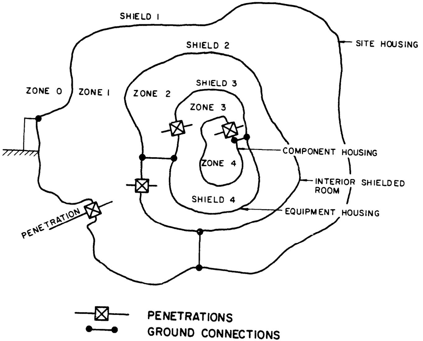
Figure 3-2. Zonal shielding concept.
